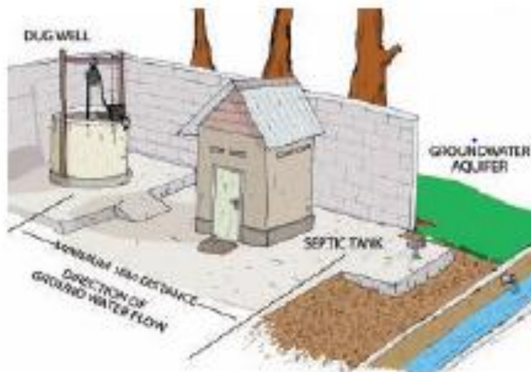
This schematic section shows the right way to site a dug well in relation to septic tank
